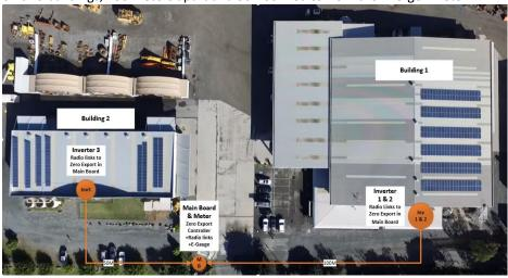
SmartConsult with its partners and engineers created a solution that allows for multiple arrays and up to 32 inverters to be control by the Supply Partners Zero Export & Inverter Ramping and provide comprehensive monitoring using an e-Gauge; all from one central point using dedicated Wi-Fi & 433 Hz radio links.
